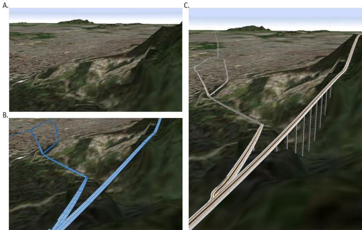
**Figure 4. A) DTM and DSM of Bogota, B) Integration between Road , DTM and DSM of Bogota, C) Highway generated by CGA.**
